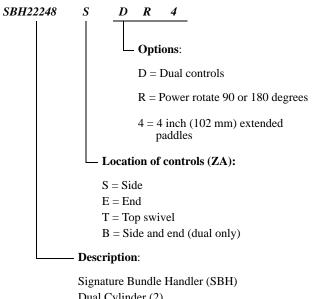
Dual Cylinder (2) WT = Weightless Top Swivel Handle 2P = Safety Interlock
